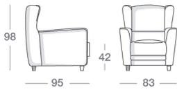
One-piece frame in double-panelled fir and poplar. **Feet in walnut-stained beech, natural sand-blasted or dark brown sand-blasted.** Differentiated density polyurethane foam filling. Springing with woven elastic straps of covered rubber. Seat cushions in differentiated density polyurethane foam with acrylic fibre covers. Decorative piping in the same shade of leather; **the piping is available on request in the other leather shades indicated in the catalogue.**
