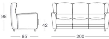
One-piece frame in double-panelled fir and poplar. **Feet in walnut-stained beech, natural sand-blasted or dark brown sand-blasted.** Differentiated density polyurethane foam filling. Springing with woven elastic straps of covered rubber. Seat cushions in differentiated density polyurethane foam with acrylic fibre covers. Decorative piping in the same shade of leather; **the piping is available on request in the other leather shades indicated in the catalogue.**
