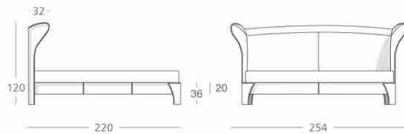
Plywood panel frame. Structural feet in plywood panel covered in same leather as bed. Differentiated density polyurethane foam filling. Decorative piping in the same shade of leather.
