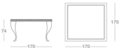
Structure in tubular steel covered in leather. **Top covered in glass, mirrored glass or in leather.** Legs in shell cast brass. Hand polish, satin-finish nickel colour, rust protection finish with clear matte enamel and wax finish.
