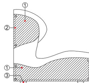
**Structure** Injected flame-retardant foam ① over internal steel frame ②. Feet ③, screwed to the frame, in black polypropylene.
